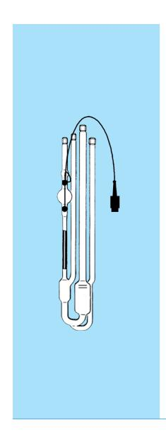
Viscometers with suspended ball level for determination of absolute and relative kinematic viscosity of liquids with Newtonian flow behaviour. The measuring levels are marked by TC sensors. The meniscus passage is detected due to the different conductivity of the liquid phase and the gas phase. A measurement stand of the type series AVS/S is not required. TC viscometers can be used to determine the kinematic viscosity of all liquids with Newtonian flow behaviour.
