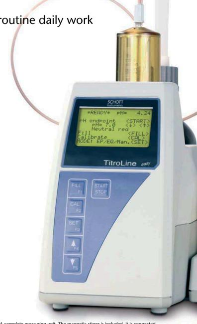
Practical and compact: A complete measuring unit. The magnetic stirrer is included. It is connected to the TitroLine *easy*. The bottle set must be ordered separately as an accessory.
