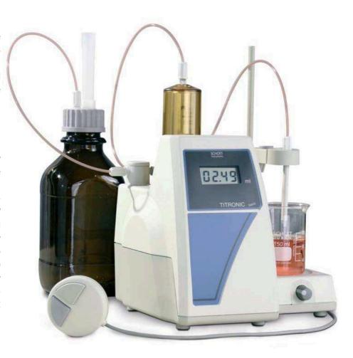
The complete workplace: precision analysis with no shaky compromises. With 8000-step resolution, precision glass cylinder with UV-protection, motor-controlled 3/2-way valve of extremely resistant PTFE/ETFE and an interface for documentation of the results. It's better to be on the safe side! (The bottle set must be ordered separately as an accessory.)
