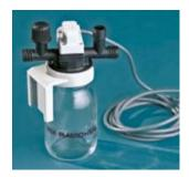
Unit with condensate trap and non-return valve with attachment for Rotavapor (not necessary with V-700 in stand-alone system).
