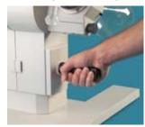
Simple raising and lowering of the flask by hand - makes operation quick and safe.
