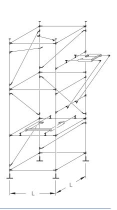
Support structures must be sufficiently rigid to prevent any bending of the individual tubes in excess of the permissible amount and the subsequent transfer of external stress to the glass components. This is achieved by incorporating additional bracing
