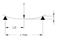
Permissible structure tubing load as a function of unsupported length
