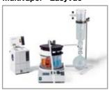
No-frills straightforward solution for automatic distillation with EasyVac (V-801). No pressure display, no sec. condenser.
