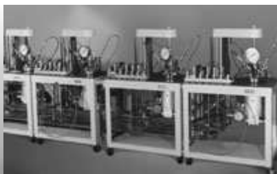
Four Interconnected Stirred Reactors with a Pressure Feed System and Full Controls Provided by Two Parr Process Controllers
