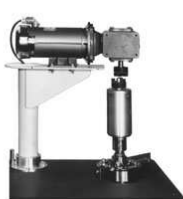
Geared Drive Motor with Cover Removed
