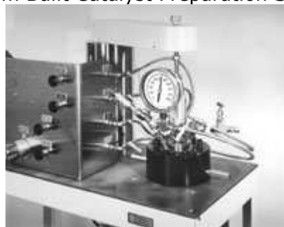
Custom Built Gas Delivery System with Flow Control Metering and Back Pressure Maintenance
