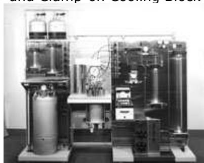
Custom Built Catalyst Preparation System
