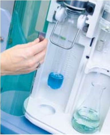
Protective door monitored by a sensor
