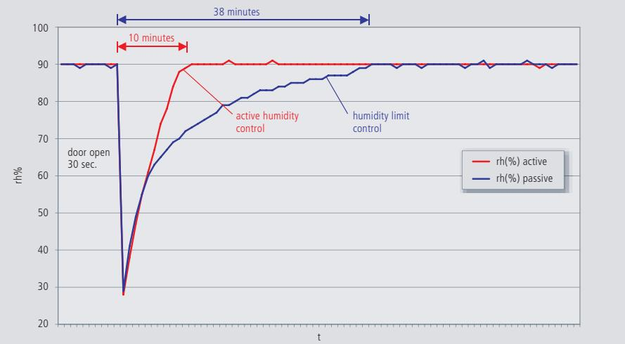
The difference in humidity recovery time between humidity limit control and active humidity control (example: INCO 2/108).
