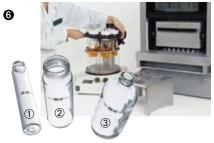
The flexible sealing system in the Multivapor makes it possible to individually seal all three collection bottles (60, 220 and 240 ml). Cross-contamination is therefore excluded.
