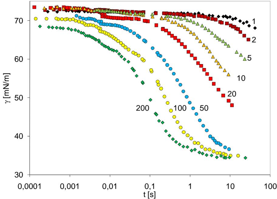
Dynamic surface tension for  $C_{14}EO_8$  solutions as a function of the effective surface lifetime. The surfactant concentrations are given as multiples of the CMC
