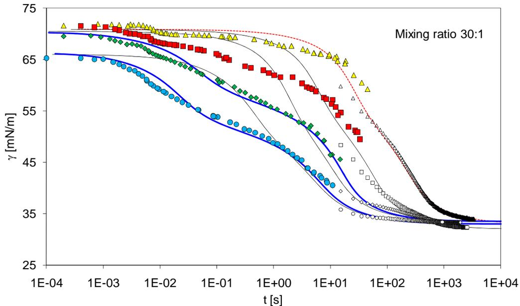
Dynamic surface tension of mixed SDS/ $C_{12}EO_5$  solutions for different molar ratio of components 30:1 and total solution concentration (top to bottom): 0.2 mmol/l (pre-micellar solution, CMC = 0.25 mmol/l); 0.5; 1.0 and 2.0 mmol/l.
