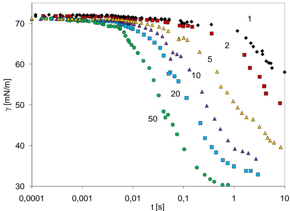
Dynamic surface tension for Triton X-45 solutions as a function of the effective surface lifetime. The surfactant concentrations are given as multiples of the CMC.
