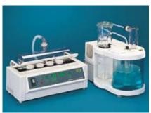
The Scrubber B-414 may also be combined with the Wet Digester System B-440 for pro-environmental preincineration of sulfate ash determination.
