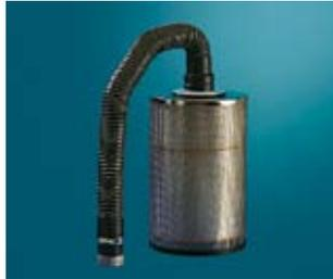
Contaminants such as particles of dust, pollen or soot are filtered out of the air entering the equipment. It is an ultra filter made of glass fiber cloth, having an effective filtering surface area of 2.3 m<sup>2</sup>.
