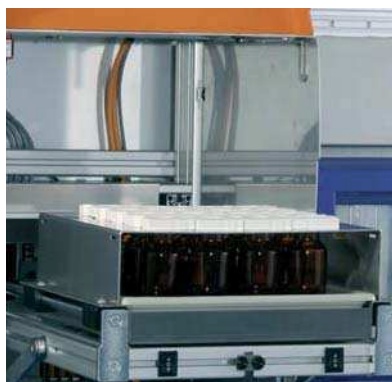
The electric sample lift ensures positioning of the samples in the rack at a convenient and easily monitored working height.
