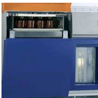
b) one rack with 16 positions to accommodate 100 ml sample bottles for normal volume applications
