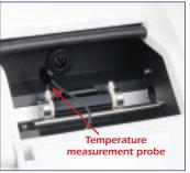
Rudolph provides a temperature validation cell with every TempTrol system. The temperature polarimeter and cell to ±0.2°C.
