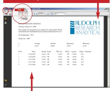
Capable of making multiple measurements on a single sample and reporting complete statistical data and all measurement results
