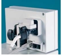
Thanks to the integrated ventilation valve the evaporation can be stopped at any time at the press of a button. The valve is open when not powered so that overpressure in the system is prevented. Only PEEK and Kalrez® materials are used to ensure the highest possible chemical resistance.
