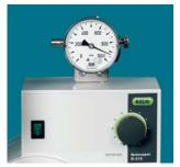
Setting of using a needle valve with simple display. For use in combination with vacuum Woulff bottle.
