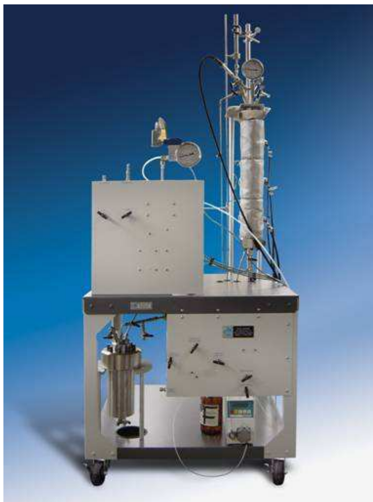
Tubular Reactor System on Floor Stand with 3-zone flexible mantle heater, one mass flow controllers, one liquid pump, and high pressure gas/liquid separator
