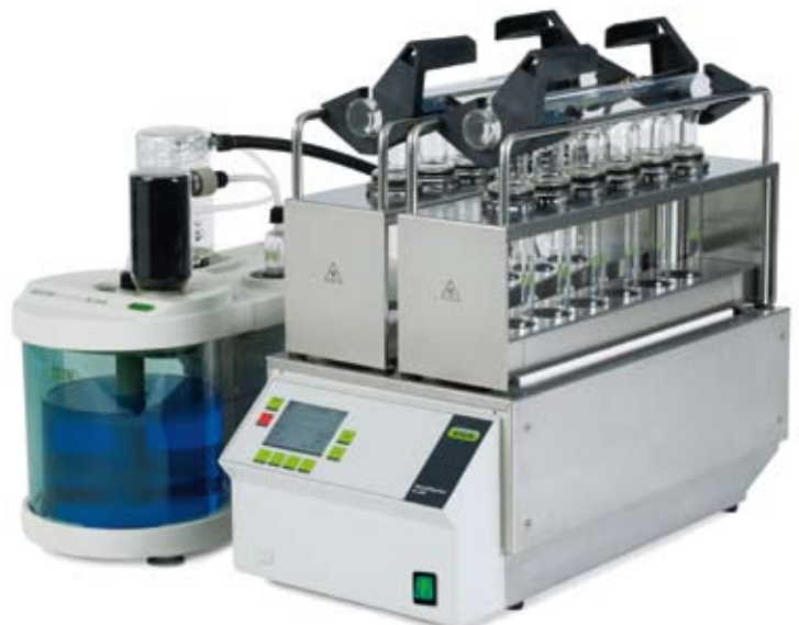
SpeedDigester K-439 with Scrubber B-414
