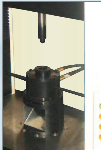
Metal piece cupping test accessory
